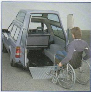
This Escort van conversion allows access and travel in the rear section for chairbound people. The rear of the vehicle is lowered via a pushbutton control to provide easy ramp access. The wheelchair locks securely into position behind the driver and up to three passengers. This stylish conversion qualifies for zero VAT rating on new vehicles.
