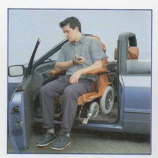
There are also systems available to allow a disabled passenger or driver to travel in their wheelchair to eliminate the problems of transfer and stowage. This design shows a lifting mechanism which picks up and transfers the wheelchair complete with occupant to lock automatically into a normal front seat position.
