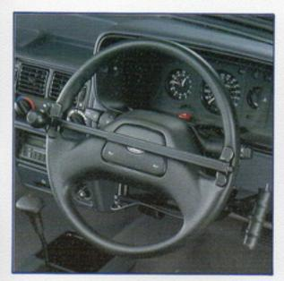
The simplest and most widespread steering aid is a knob or spinner fitted to the existing steering wheel. This is needed by anyone steering with only one hand, but is also helpful for someone with a weak grip. Another common type of control is the conversion of both brake and accelerator to hand operation. Hand controls are usually fitted in combination with automatic transmission.
