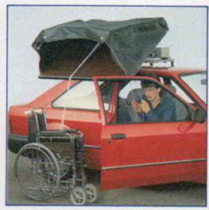
Someone who is less agile could consider a car-top hoist and stowage system which involves less effort and physical movement to use. This equipment collects a wheelchair from the side of the car, holds it securely in transit and returns it to your side at the end of a journey. The controls are designed for automatic operation from inside the car.
