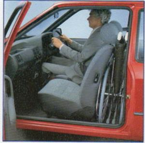
Motoring with a wheelchair brings a new set of problems which can be overcome in a variety of ways. Some wheelchair users are able to get into their cars and store their wheelchairs without assistance. This may involve stowing and retrieving the wheelchair from the car boot or load compartment or pulling it into the car after you. The 2 door Escort is particularly well suited to this method of 'drag-in' storage because of its wide doors and ample space between the front and rear seats.
